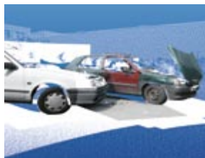
Point clouds with true-color rendering assist in capturing accident or damage data for forensic analysis and court reference.
