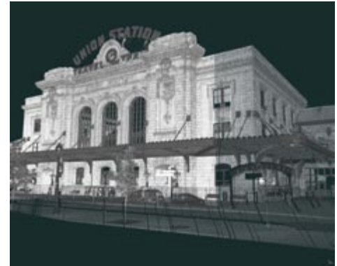
Grey-scale intensity additional viewing mode. Ideal for 2D drawing over orthophotos.
