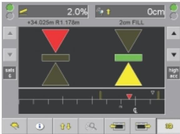
The **Cross-section View** screen displays a cross-section of the design at the operating elevation and the current location. The operator can zoom the display in or out simply by touching the screen.
