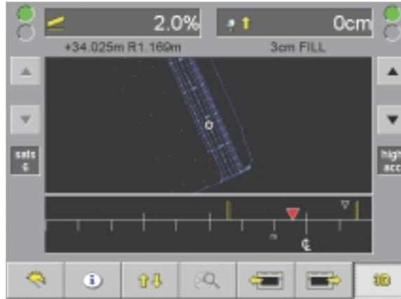
The **Data View** screen displays position information to ensure that the system is set up correctly; this view also aids in troubleshooting.
